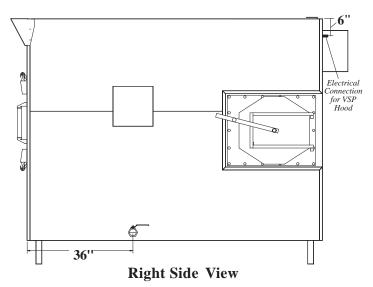
**Electrical Requirements:** 120 volts AC, 60 hertz, 1 phase, 15 amp wiring required.
