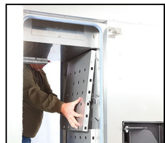
Removal of Air Channel
