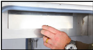
Convection blower wheel access for inspection/cleaning.
