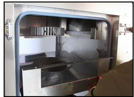
Removing shroud provides complete access to convection blower wheel for cleaning and/or removal of blower wheel.
