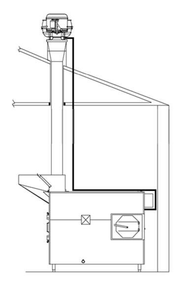
A STANDARD TOP EXHAUST APPLICATION IS SHOWN HERE. CONNECTIONS ARE THE SAME FOR OTHER MODELS. FANS REQUIRING ABOVE 120V POWER CANNOT BE POWERED BY SMOKER. IF POWER GREATER THAN 120V IS REQUIRED, CONSULT FACTORY.
