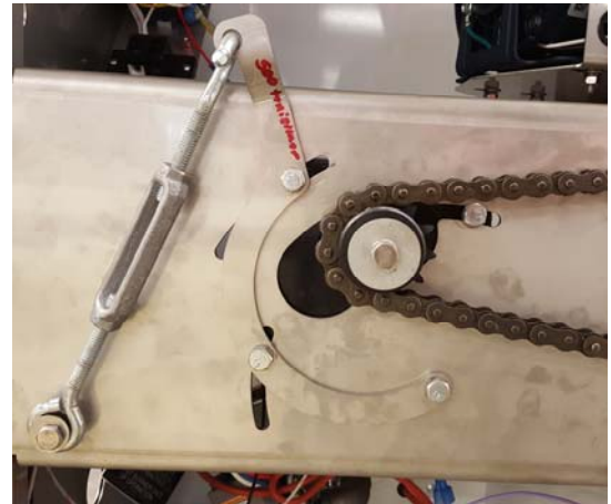
New Turnbuckle Style Chain Tensioner
